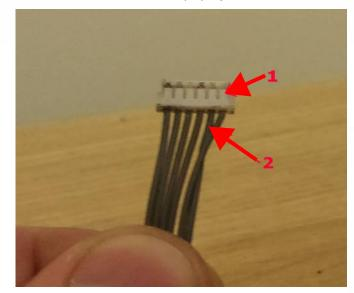
Lift plastic tab (1) with knife edge or small tip screwdriver and pull wire out . Now swap it with the wire in the second position (2) using the same method. Next, crimp the plastic tab back down with needle nose pliers. Gently tug on the wire to make sure they are secure.
