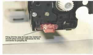
If the drum doesn't smoothly slide into place, don't force it. Forcing it could damage/push out the connector on the machine side. Just file the connector down a little more until it fits properly.
