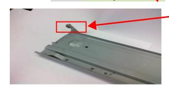
Cut the pin at the rear of the base plate so it is flush with the top of the guide rail.
